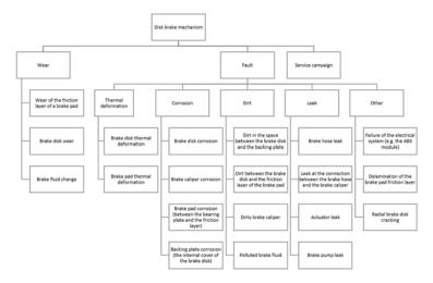
*Fig. 4. Types of interventions concerning repair or replacement of disc brake components in the studied units*
