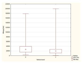
Fig. 14. Box plots of the mileage distribution of the vehicles reported due to a fault for brands X and Y
