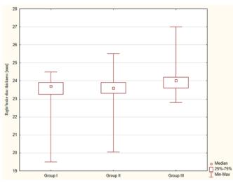
Fig. 13. Box plots of the distributions of the right disc thickness in the vehicles reported due to wear in groups of vehicles with different body types
