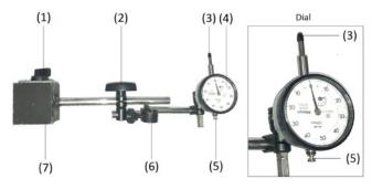
*Fig. 2. A dial indicator for measuring the deformation level of brake discs on a magnetic stand*
